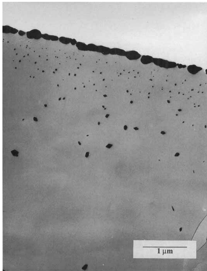
Figure 5 Transmission electron micrograph of the surface of the 17% gold auric acid doped BTDA/4-BDAF film.
